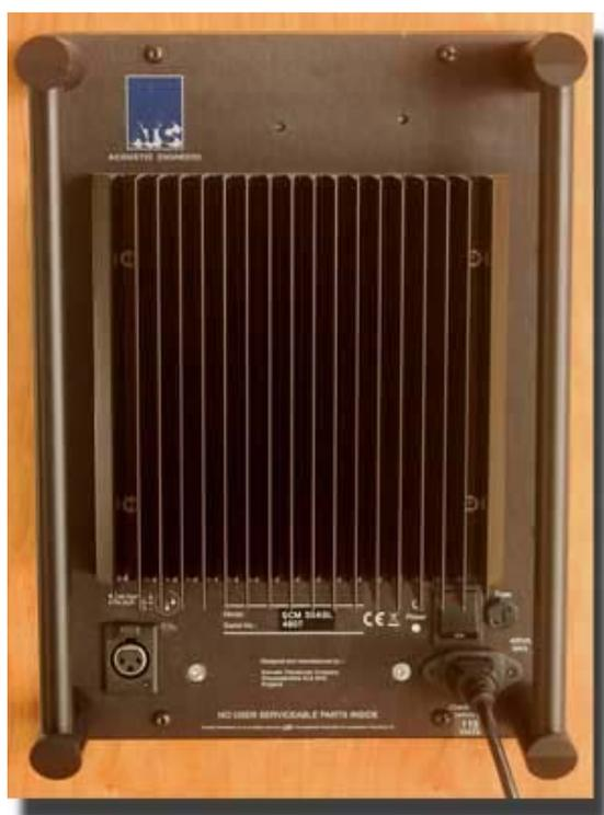
Being self powered, the ATC's employ built in amplification called the "Ampack" previously mentioned. Woodman told me that the Ampack incorporates phase correction and momentary gain reduction to prevent clipping the amplifiers when listening to very loud music when the output stage is driven to near full output. Bulletproof. The power stage of the amplifier is of a ground source MOS FET design and operates in class AB.
