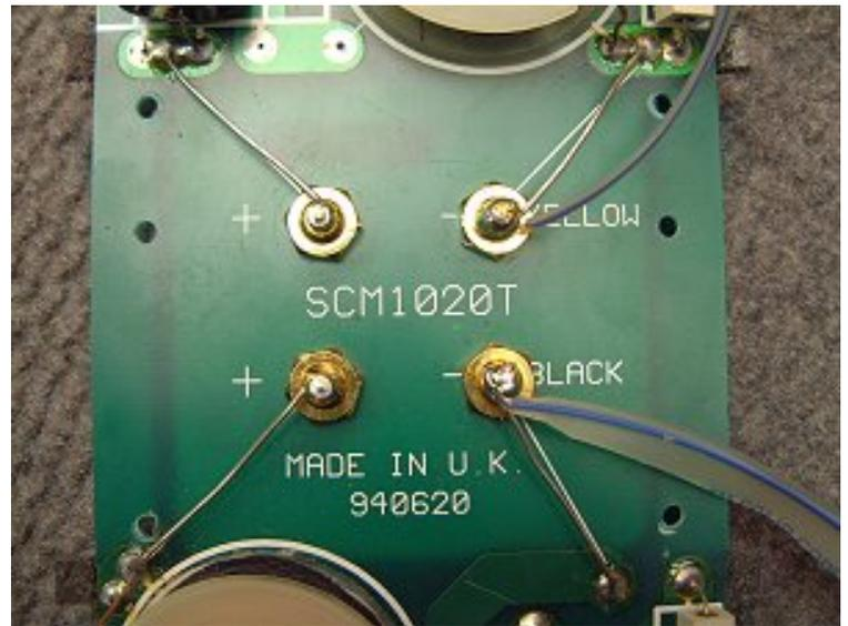
The bass and treble sections of the crossover are shown here. The bass path is a simple 12dB/octave LC filter, with an RC impedance-correcting network in parallel with the drive unit. For the treble, a similar LC filter is followed by a resistive T-section attenuator to bring the tweeter level down to match the woofer.
