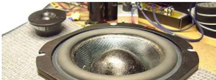
to a woven cone and 3 inch soft dome, both of which are hand-doped with a rather sticky damping material.
