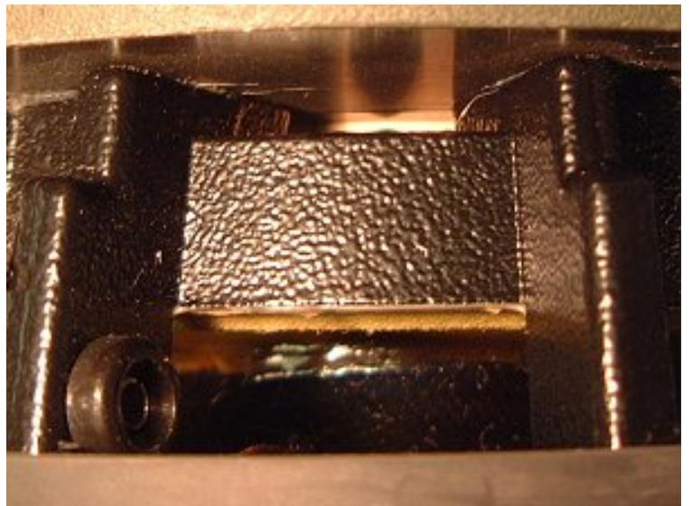
The tweeters are supplied by Vifa, and use a conventional 1 inch soft-dome. The thick aluminium faceplate is an ATC modification, and has a short flared section which provides dispersion control. The rear of the magnet is covered by a plastic enclosure, the air contained within playing a part in the acoustic performance, thanks to a vented centre pole-piece. While somewhat overshadowed by the bass driver, it certainly feels like a high quality device...
