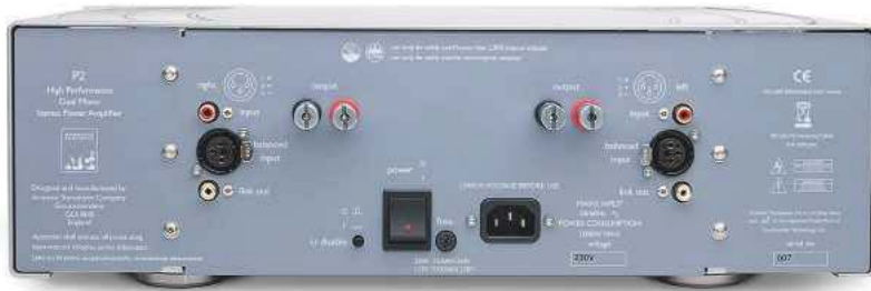
ABOVE: Single-ended (RCA) and balanced (XLR) inputs are joined by single-ended loop-through outputs and a single set of unswitched 4mm speaker binding posts
