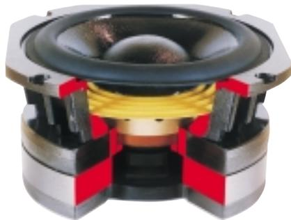
Super Linear Magnet Material (SLMM) Technology, introduced in 1996, is the culmination of two years research and development by Billy Woodman into the inherently non-linear magnetic performance of soft steel, and eddy current and hysteresis distortion in driver magnet assemblies. ATC claims the result is a major breakthrough in moving coil drive unit design.
