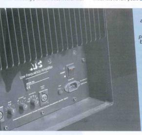
A 1kW amplifier on the C4 subwoofer provides the bottom-end muscle
