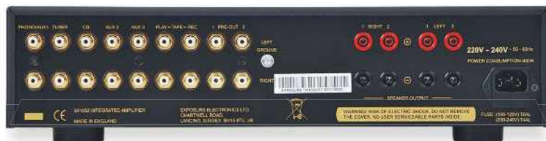
ABOVE: In addition to six RCA line inputs, the Exposure's back panel offers two sets of preamp outputs for bi-wiring, and two pairs of speaker outputs, plus IEC mains in
