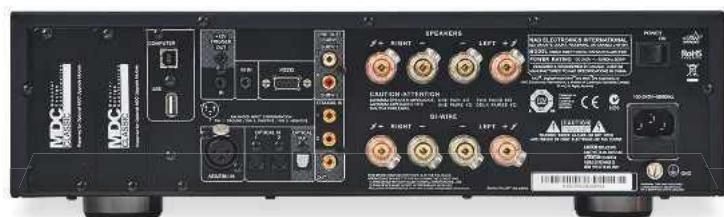
ABOVE: MDC expansion card slots sit far left, with digital inputs (AES/EBU, USB, optical and coaxial) adjacent. Two pairs of speaker binding posts take centre stage
