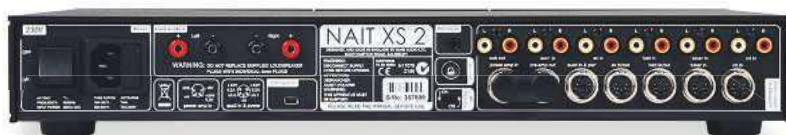
ABOVE: Crowded back panel includes USB upgrade socket, one set of speaker outputs, link plug for power supply upgrade and five RCA/DIN socket line inputs
