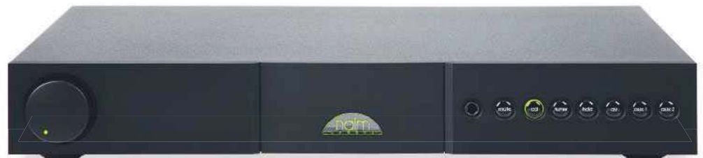
ABOVE: XS2 fascia is a model of simplicity. Unusually, volume control is far left, with illuminated Naim logo in the centre. The five source selection and mute buttons are also backlit
