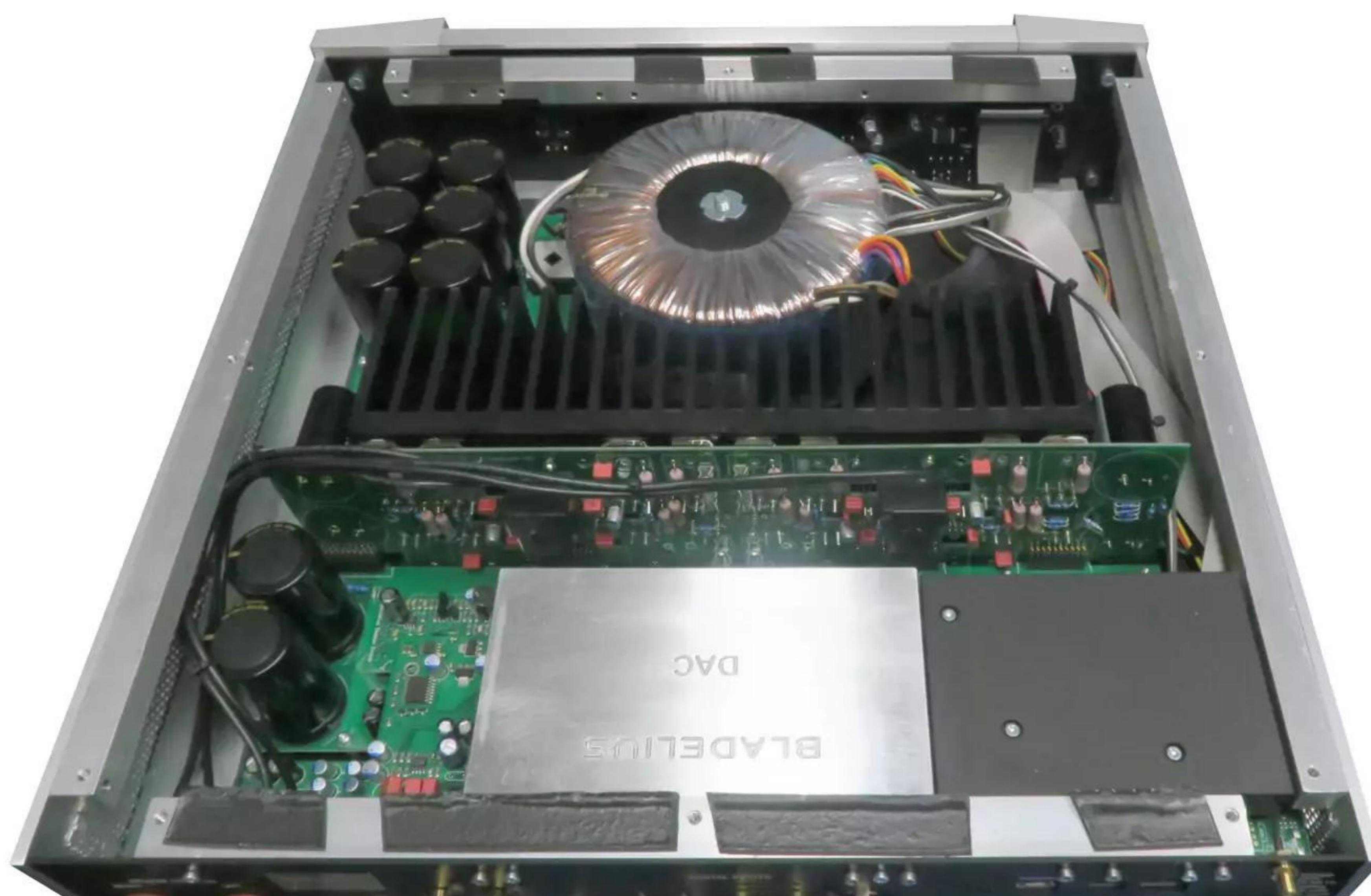
▷ THE BLADELIUS ASK'S MASSIVE 2KVA TOROIDAL POWER TRANSFORMER IS A CUSTOM-MADE BEAST
